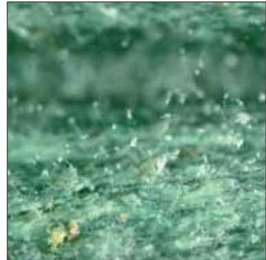
Fig. 5: Mould on test specimen 10 (H40), 40-fold enlargement.
