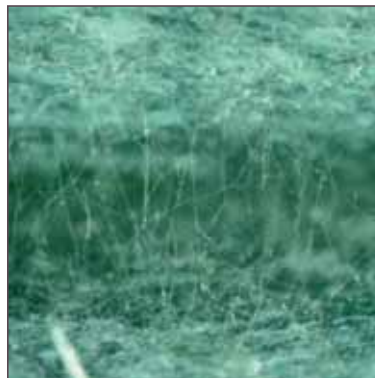
Fig. 7: Mould on test specimen 59 (H40), 40-fold enlargement.
