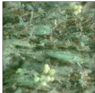
Fig. 8: Mould on test specimen 72 (H41), 70-fold enlargement.
