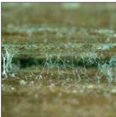
Fig. 9: Mould on test specimen 77 (Bangkirai), 50-fold enlargement.
