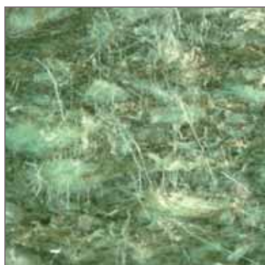
Fig. 10: Mould fungi on test specimen 122 (H41), 40-fold enlargement
