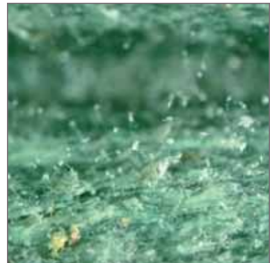
Fig. 5: Mould fungi on test specimen 10 (H40), 40-fold enlargement
