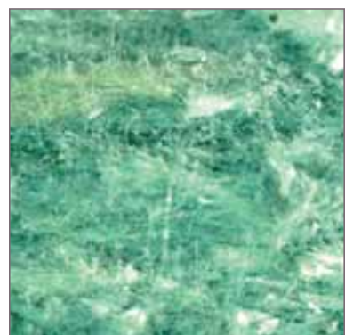
Fig. 11: Mould fungi on test specimen 161 (H40), 40-fold enlargement
